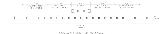
Quarter spacing (posts every 1'- 6.75") Start half post spacing 25' before hazard Start quarter post spacing 12.5' before hazard End quarter post spacing 12.5' past hazard End half post spacing 25' past hazard
